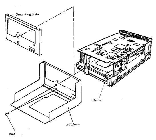
Figure 1-22. Connect the M2488 and the ACL Base
